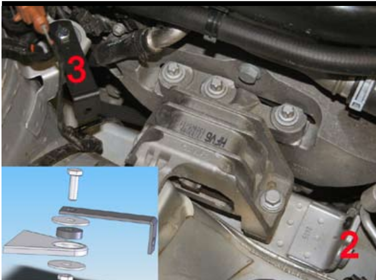
3. Mount the rubber lead-through (2) and the rod (3) with M8 screw/nut (do not tighten fully yet). Mount the washers as the picture shows.
