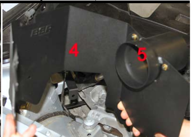
4. Mount the pipe (5) to the heat shield (4). Use M5.
