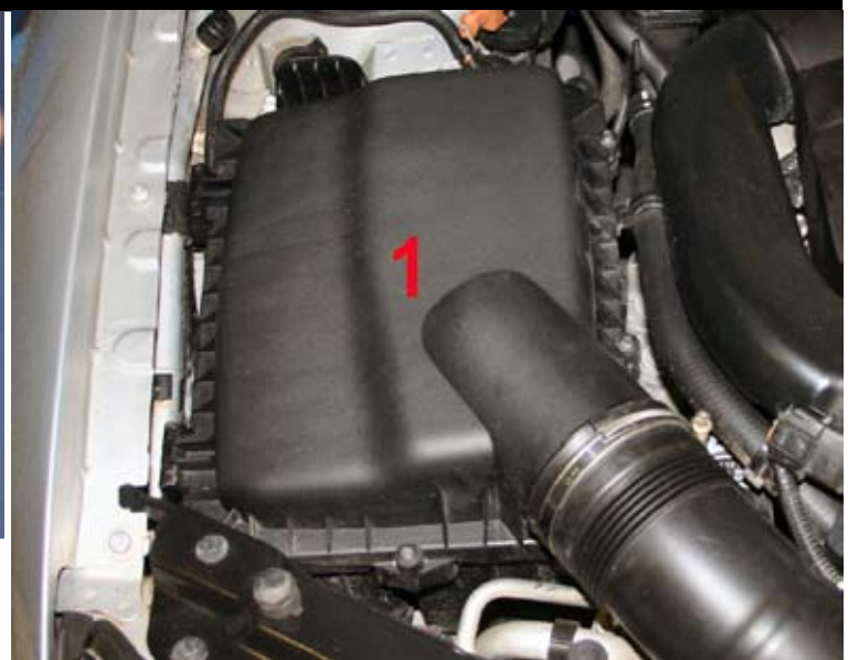
2. Remove the air filter box (1). Start with the lid. Loosen the torx screws and the hose clamp. Lift up the bottompart. (The original rubber lead-throughs is not to be used)
