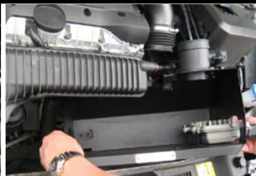
12. Assemble the OptiFlow heat shield to the car, slide it down from right to left. Fit the steering pin under the OptiFlow heat shield to the rubber bushing (See pic 11 point 6).
