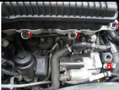
11. Assemble the plastic "washer" to the rubber-bushings (7).
