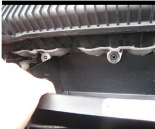
13. Tighten the heat shield, start with the two attach points to the left, leave the third for later
