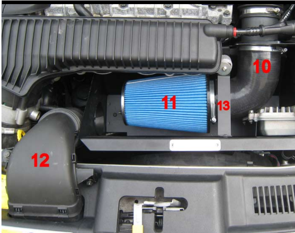
14. Assemble the harness connector and the air hose to the air mass meter. Assemble the two harness connectors to the ECU. Snap on the red locks. Assemble the vacuum pipe to the inlet.
