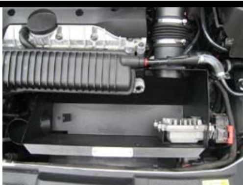
14. Assemble the harness connector and the air hose to the air mass meter. Assemble the two harness connectors to the ECU. Snap on the red locks. Assemble the vacuum pipe to the inlet.
