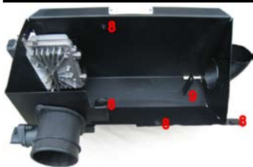
10. Assemble the 6 plastic clips to the plate (8). Assemble the air mass meter and the ECU to the OptiFlow heat shield. Assemble the rod (9). (as picture shows)
